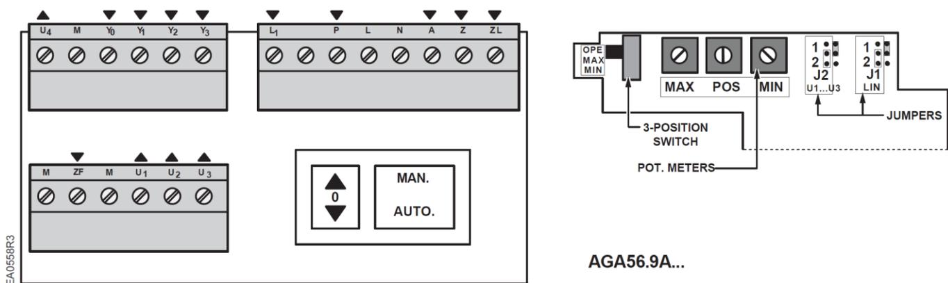
**Figure 12. AGA56.9... Terminal and Trim Potentiometer/Jumper Board.**
